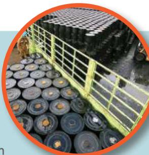
Asphalt is one of the building materials that is used in a road construction or circulation project, has its main function as a binding agent and cladding of ground surface which applied by mixing another compounds such as bitumen and mineral. Asphalt will bind these components to be attached to rocks and other components in to the road surface.
